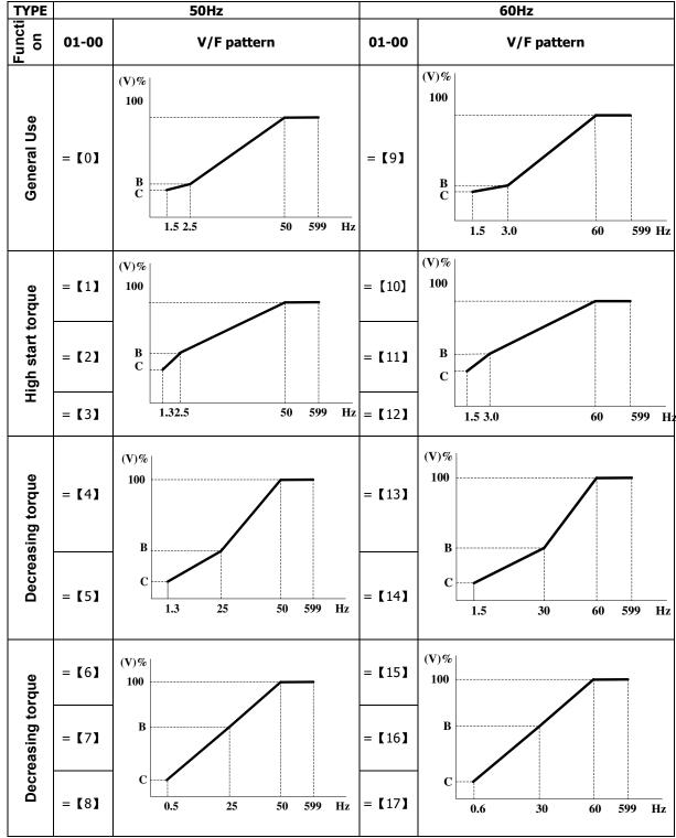
(V) 100% is the maximum output voltage. B, C point preset % settings will be as table below:
