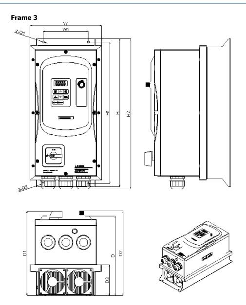
Figure 4-9: dimensions frame size 3
