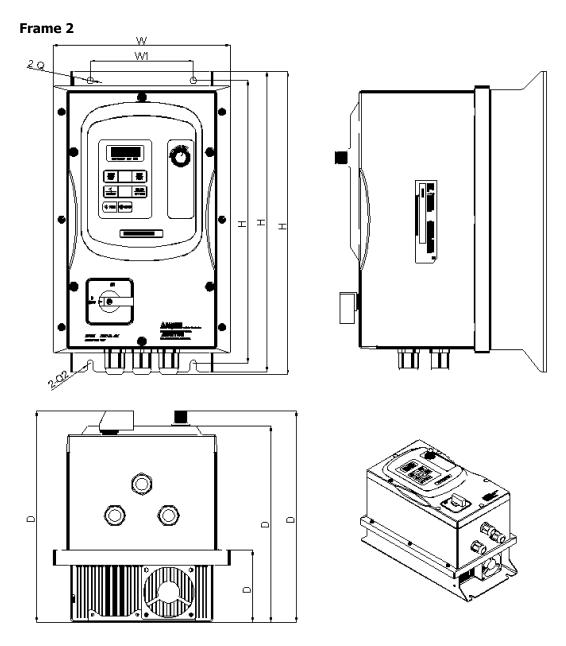
Figure 4-8: dimensions frame size 2
