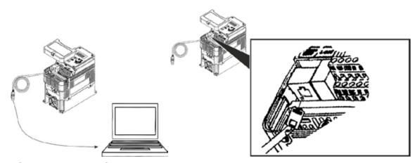
Figure 9-2: connecting to PC
