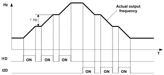
Mode 2: If UP or DOWN input terminals are turned on for more than 2 sec, the original UP/DOWN mode is restored output frequency ramps up or down as long as the input is kept ON.
