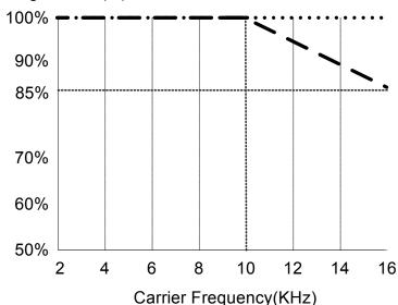
Note: De-rate curve for ambient temperature of 40 degree C.
