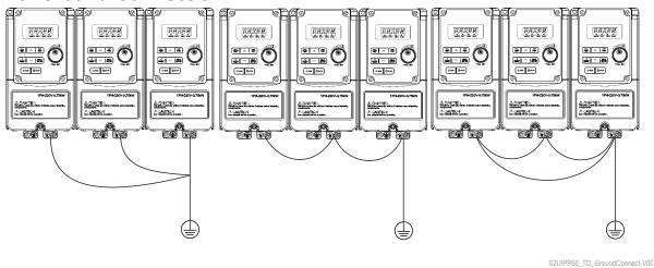
(a) Correct (b) Correct Figure 7-2: ground connection wiring example
