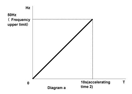
Diagram a: Target frequency is determined by the Frequency upper limit, the on-time and accelerating time 2.
