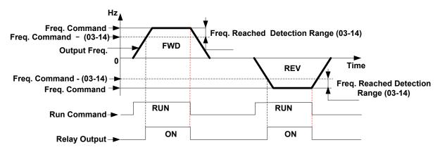
Example: Freq. command=30 Hz and 03-14=5 Hz. Relay turns ON when output freq. reaches 25 Hz to 30 Hz.
