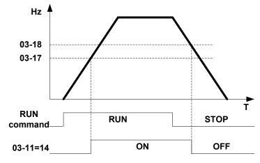
Timing diagram for  $03-17 \ge 03-18$  is shown below:
