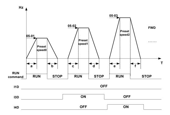
When the run command is On/Off, acceleration and deceleration times for each cycle can be calculated as below:- time unit is in seconds.
