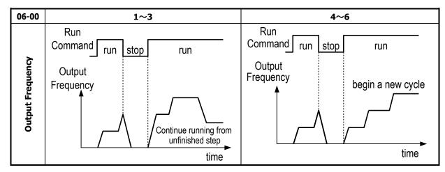
ACC/DEC time in Auto run mode will be according to the setting of 00-14/00-15 or 00-16/00-17.
