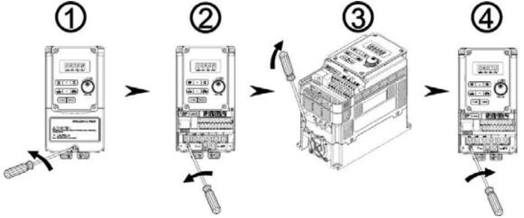
Figure 7-6: disconnecting the EMC filter
