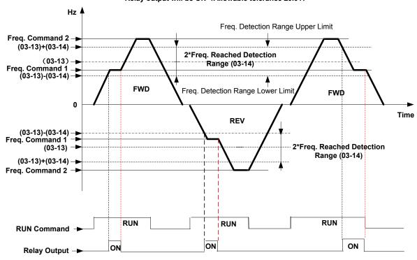
5) 03-11= 【4】. RY will be on as soon as the Output frequency > Preset frequency reached level (03-13)
