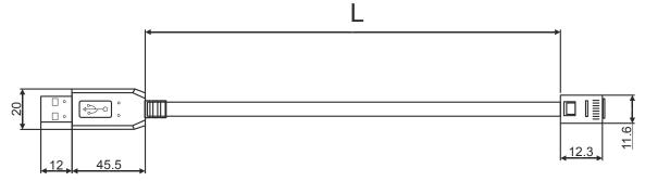
Figure 9-1: connecting cable (dimensions in mm)
