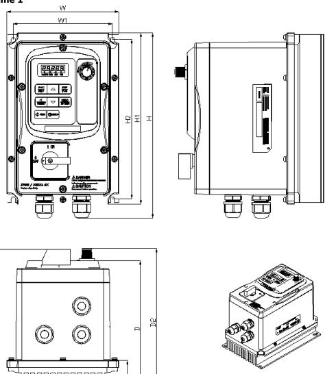
Figure 4-7: dimensions frame size 1
