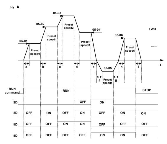
When the run command is continuous, acceleration and deceleration times for each segment can be calculated as below:
