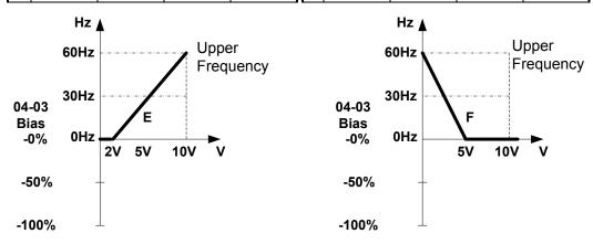
**3) Offset bias** set to 0% (04-03) and effect of modifying Analog Gain (04-02), Bias type (04-04) and slope type (04-05) are shown in shown Fig 5&6.
