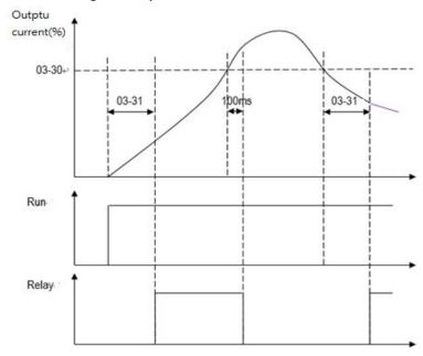
When **03-29= [1]**, if output current lower than low current detection time (setting value of 03-30), relay will be closed by lower current detection time (setting value of 03-31). (There is a 0.6 s sampling delay time at power on)
